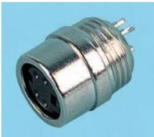
An S-Video type (4-pin MiniDIN) socket with solder bucket terminations. Supplied with fixing nut. Panel cutout: Ø11mm approx.
