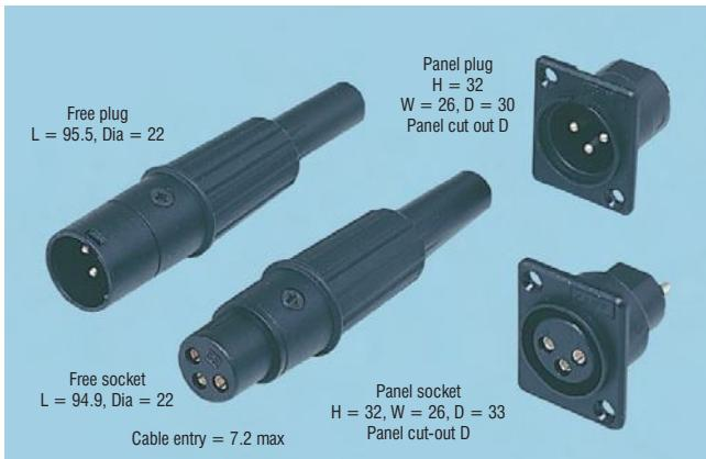
A range of lightweight yet robust, black plastic and audio connectors. Suitable for speaker connection or any other applications where screening is not essential. The free plugs feature a snap fit cable clamp/strain relief which substantially speeds up connector assembly time.
