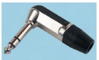
General purpose 90° 6.35mm (1/4") jack plugs featuring crimp strain reliefs and available with nickel plated contacts. Maximum cable diameter 6mm.
