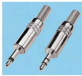
All metal Jack plugs with chrome plated metal bodies and nickel plated contacts. The plugs also feature spring cable strain reliefs and accept cables up to Ø5mm.
