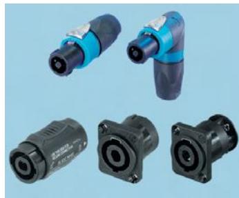
Meeting the requirements of all major broadcasting authorities, these rugged, 'Quicklock' latching 4-pole connectors are for professional loudspeaker/amplifier interconnections. For ease of assembly, all terminations are solderless. The chassis socket is airtight, and fits cut-outs for existing audio connector types. The coupler enables in-line connection of two plugs for cable extensions.
