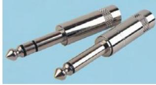
General purpose 6.35mm (1/4") jack plugs featuring crimp strain reliefs and available with nickel plated contacts. Maximum cable diameter 6mm.
