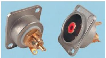
High quality D mount phono sockets designed to fit standard 24mm D type cut-outs. Featuring gold plated contacts and are available with red or white inserts.
