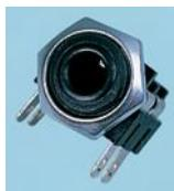
Mono jack sockets for front panel mounting with switching action on insertion of a 3.5mm jack plug. Solder tag connections.
