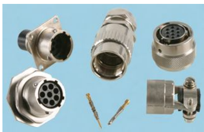
Metal circular connector with metal bayonet coupling system.
