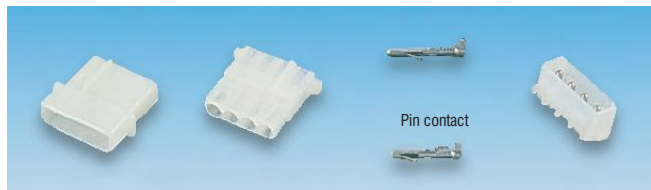
Pin housing Socket housing Socket contact PCB pin header PCB mounting centres 4 x 1.78 dia, 5.08 (0.2") Pitch
