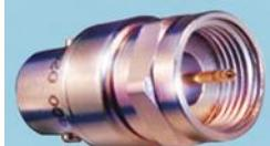
Twinaxial and triaxial connectors are concentric designed with 2 concentric contacts which are isolated from each other, the middle contact and the shielded terminal. They are used in digital data buses, MIL-STD-1553B base band circuits and video pair applications. The connectors do not need mechanical alignment.
