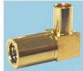
SSMB connectors are microminiature devices that provide repeatable electrical performance from DC up to 4 GHz. They are a smaller version of the standard SMB connector, providing a means of quick-connect and disconnect through a snap-on type coupling.
