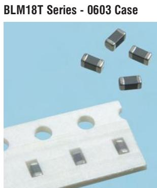
The chip ferrite beads BLM series is designed to function nearly as a resistor at noise frequencies, which greatly reduces the possibility of resonance and leaves signal wave forms undistorted.
