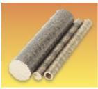
Leaded Gunmetal SAE660 is a general purpose bearing alloy containing tin, lead and Zinc giving a good all round balance of properties of strength, hardness, machinability and abrasion resistance which makes it ideal for the fabrication of bearings and bushes.
