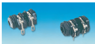
148-266 (Panel) H=23.8, W=20.4, D=21.3 Panel cut-out=11.0 dia (plastic nut) 11.5 dia (chrome nut), Pins=solder lug type
