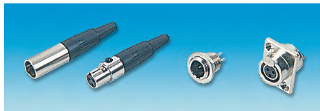
Free plug L = 51.7, Dia = 10.5 Cable entry = 3.0 dia Free socket L = 48.3, Dia = 10.5 Panel plug Cut-out = 11, D = 17.5 Panel thickness = 7 max. Panel socket Cut-out = 15.2 Fix. cent = 17.1 11.4 H = 24.4, W = 18.8
