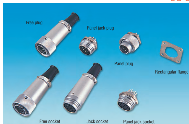
Free plug L = 51.7, Dia = 10.5 Cable entry = 3.0 dia Free socket L = 48.3, Dia = 10.5 Panel plug Cut-out = 11, D = 17.5 Panel thickness = 7 max. Panel socket Cut-out = 15.2 Fix. cent = 17.1 11.4 H = 24.4, W = 18.8
