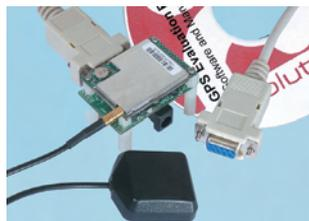
The LS range of GPS modules are compact solutions intended for a broad range of products, where fast easy system integration and minimal development risk is required. The receiver continuously tracks all satellites in view and provides accurate satellite positioning data. They are suitable for a wide range of OEM configurations including handhelds, sensors, asset tracking, PDA-centric personal navigation system, and vehicle navigation products.
