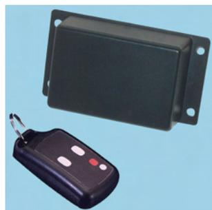
A versatile general purpose remote control, which can be used for controlling many different applications. The system utilises a highly secure Code Hopping protocol to ensure reliable operation.
