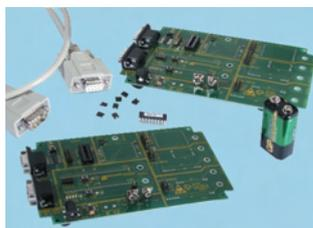
The Smart Radio Evaluation Kit provides a hardware platform to enable fast development of radio applications.
