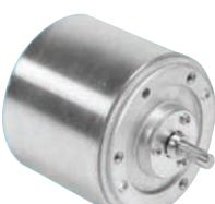
The M66CE is a high performance low inertia dc servo motor, providing high output power and offers smooth operation over a wide speed range. The M66CE motor incorporates a skewed ironless rotor thereby ensuring linear speed and torque characteristic combined with rapid acceleration and reversal capabilities. There is a 17mm long rear shaft of 4mm diameter and a 24mm long front shaft of 6mm diameter. The 2 connecting wires are approximately 235mm long.
