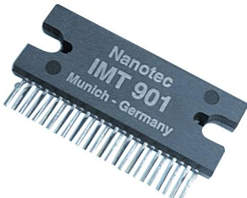
The IMT 901 is a PWM chopper type sinusoidal micro step bipolar stepping motor driver. Sinusoidal micro step operation is generated by means of built-in hardware and is outputted for operation by clock signal inputting.
