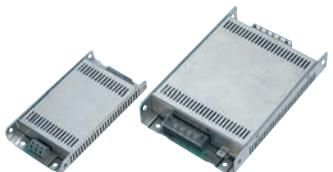
Motor inverter high performance filters designed to enable inverters to meet the most stringent **EMC** limits as laid down in **EN55022B**. Flexible mounting options ensure minimal canel space occupation. Finger proof terminals are used up to 30A and insulating boots cover stud terminals above 30A. Designed to meet the requirements of **IEC950**.
