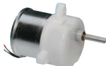
The B138F features a durable spur gearbox in a 34mm-diameter moulded-plastic housing with three-point mounting built-in for straightforward installation. A wide range of standard reduction ratios is available, from 12.25:1 to 1470.82:1, with maximum output torque from 1.5 to 50Ncm.
