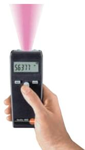
Using the Testo 465, rpm can be easily measured optically without contact. Simply attach a reflector to the object to be measured and point the visible red modulated light beam at the reflector and take a measurement.
