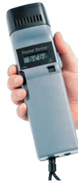
The testo 476 Pocket Strobe™ hand-held stroboscope measures and checks rotation and vibration movements. It facilitates the measurement of very small objects or in hard-to-access places. The energy optimised switching electronics and light-intensive xenon flash lamp facilitate a high light intensity (approx. 800 lux).
