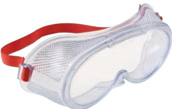
A range of goggles with a wide vision area, made from soft PVC. Contoured PVC body, Polycarbonate Lens. Direct vent goggle. Conforms to EN166.1B.
