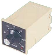
An electronic relay that gives an output when the rotation of a machine shaft ceases. Inputs from a 3-wire inductive proximity sensor, determined by the speed of shaft rotation, resets a timer within the sensor and prevents the output contacts from energising. Potentiometer control for time delay 1 to 30 secs. If a pulse is not received within the set period the sensor energises and an LED indicates the shaft has stopped.
