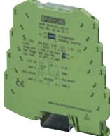
3-way isolating amplifier for the electrical isolation of analogue signals, I/O can be configured via DIP switches, with screw connection.
