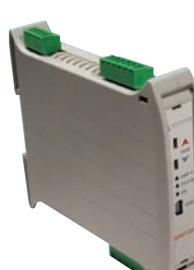
This new generation of signal conditioner has been designed to accept most common process and temperature sensor inputs and provide the user with a programmable current or voltage output signal plus dual relays with a programmable delay function. 3 way isolation is provided and all temperature ranges are linear to temperature. Both input and output loop excitation is provided as well as a fully universal power supply.
